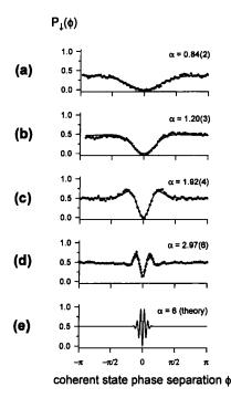
Figure 8.  $P_{\perp}(\phi)$  interference signal with increasing values of  $|\alpha|$ . The data are fitted to equation (10), yielding  $\alpha = 0.84$ , 1.20, 1.92 and 2.97. The fit in curve (d) includes a term to account for the loss of contrast.
