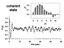
Figure 4.  $P_{\downarrow}(t)$  for a coherent state, showing collapse and revival. The data are fitted to a coherent state distribution, yielding  $\bar{n} = 3 \cdot 1 \pm 0 \cdot 1$ . The inset shows the decomposition of the data onto the expected Fock state components, fitted to a Poissonian distribution, yielding  $\bar{n} = 2 \cdot 9 \pm 0 \cdot 1$ .
