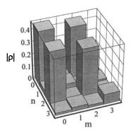
Figure 12. Reconstructed density matrix amplitudes of an approximate  $1/\sqrt{2}(|n=0\rangle - i|n=2\rangle)$  state. The state was displaced by  $|\alpha| = 0.79$  for N = 4 in equation (14). The amplitudes of the coherences indicate that the reconstructed density matrix is close to that of a pure state.
