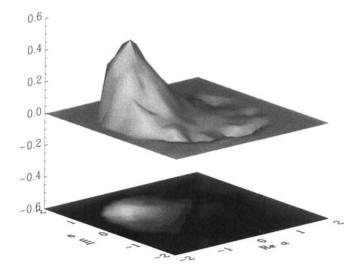
Figure 11. Surface and contour plots of the reconstructed Wigner function of a coherent state. The approximately Gaussian minimum uncertainty wavepacket is centred around a coherent amplitude of about 1.5 from the origin. The half-width at half maximum is about 0.6, in accordance with the minimum uncertainty half-width of  $[\ln(2)/2]^2 \approx 0.59$ .
