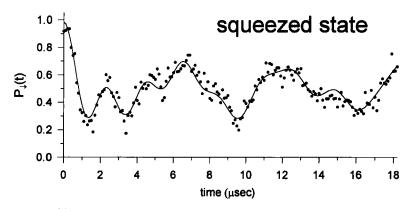
Figure 6.  $P_{\perp}(t)$  for a squeezed state. The data are fitted to a squeezed state population distribution, yielding  $\beta \approx 40 \pm 10$  (16 dB below the zero point variance), which corresponds to  $\bar{n} \approx 7.1$ .
