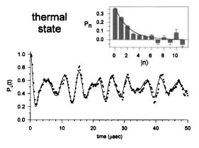
Figure 3.  $P_{\perp}(t)$  for a thermal state. The data (points) are fitted (line) to a superposition of Fock states with  $P_n$  given by a thermal state distribution. The fit allows  $\bar{n}$  to vary, yielding a value of  $1.3 \pm 0.1$ . The inset shows the decomposition of the data onto the Fock state components (bars) with a fit (line) to the expected exponential distribution, yielding  $1.5 \pm 0.1$ .
