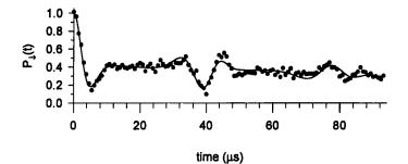
Figure 5.  $P_{\downarrow}(t)$  for a coherent state, driven on the second blue sideband. Since the Rabi frequencies are almost commensurate in this interaction,  $P_{\downarrow}$  shows very sharp collapse and revival features. The solid line is a fit using the exact Rabi frequencies for finite  $\eta$ . It yields  $\bar{n} = 2.0 \pm 0.1$ .
