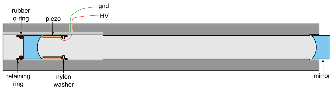
Figure C.1: Invar cavity assembly diagram. The components on the left (mirror, piezo tube, rubber o-ring and nylon washer, all held in place by two retaining rings) are assembled prior to alignment. The second mirror is initially mounted on an external optics mount that can be controllably translated along the axis of the cavity. As the cavity is scanned with light incident on the back face of either mirror, the secondary mirror is adjusted to make the cavity confocal. It is then secured with a dab of epoxy, and the external mount removed.
