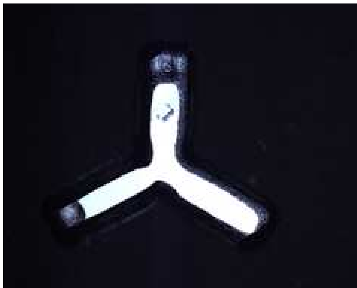
Figure 6.7: Future trap designs might include junction regions (for a three layer trap, but not a two layer trap). This junction would require a “Y” shaped backside etch, complicated by the etching differences between the axis parallel and perpendicular to the substrate flat. By aligning one stem of the Y parallel to the flat and the other stems at a 60^\circ angle, the membrane edges come out straight, similar to figure 6.3
