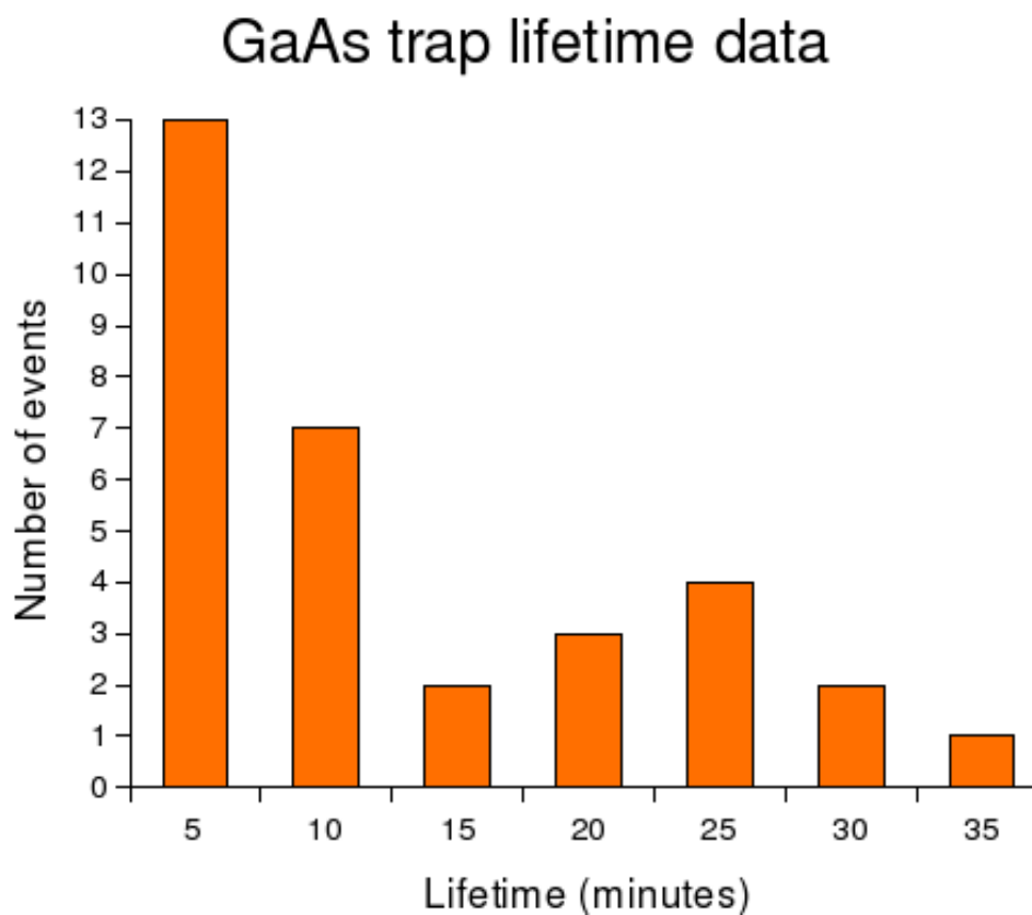
Figure 6.13: This histogram shows the lifetime statistics for 32 different ions while being continuously Doppler cooled. The events are binned into time groupings of 0-5 minutes, 5-10 minutes, . . . . The second peak at the 20-25 minute bin suggests that once an ion has survived past the high pressure period caused by the oven being fired, it is most likely to last till this 20-25 minute period. Most ions, however, do not survive this long due to a collision with a background molecule or Cd atom.
