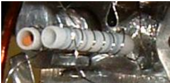
Figure 4.6: This figure shows two cadmium ovens, made out of a ceramic tube with tungsten wire coiled around each tube for heating them. The red material seen on the inside is cadmium oxide. Typically an oven like this would also have a small ceramic aperture at the front to make sure the cadmium oxide does not fall out.
