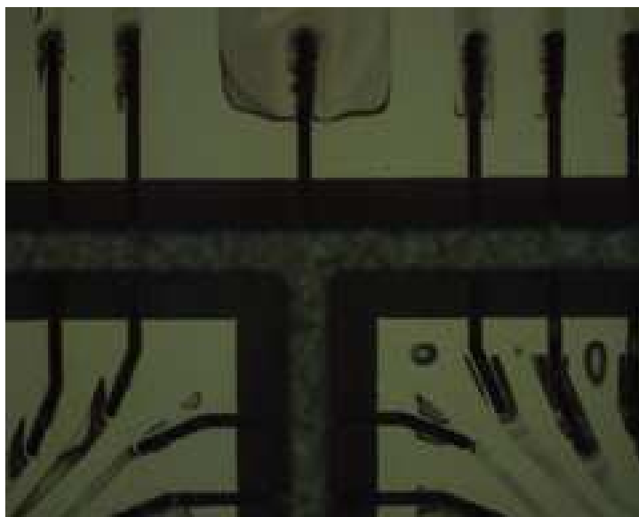
Figure 5.6: Since the photoresist had to stay in longer to develop the edges and cantilevers (you can still see some on the right corner cantilever), some of the photoresist between two wires came off (see the left corner cantilever).
