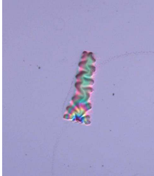
Figure 6.6: This image of the MBE grown membrane after the back-side has been etched shows it buckling under the strain from the substrate. When the cantilevers are etched in the ICP this strain will be relieved and the cantilevers will be flat.
