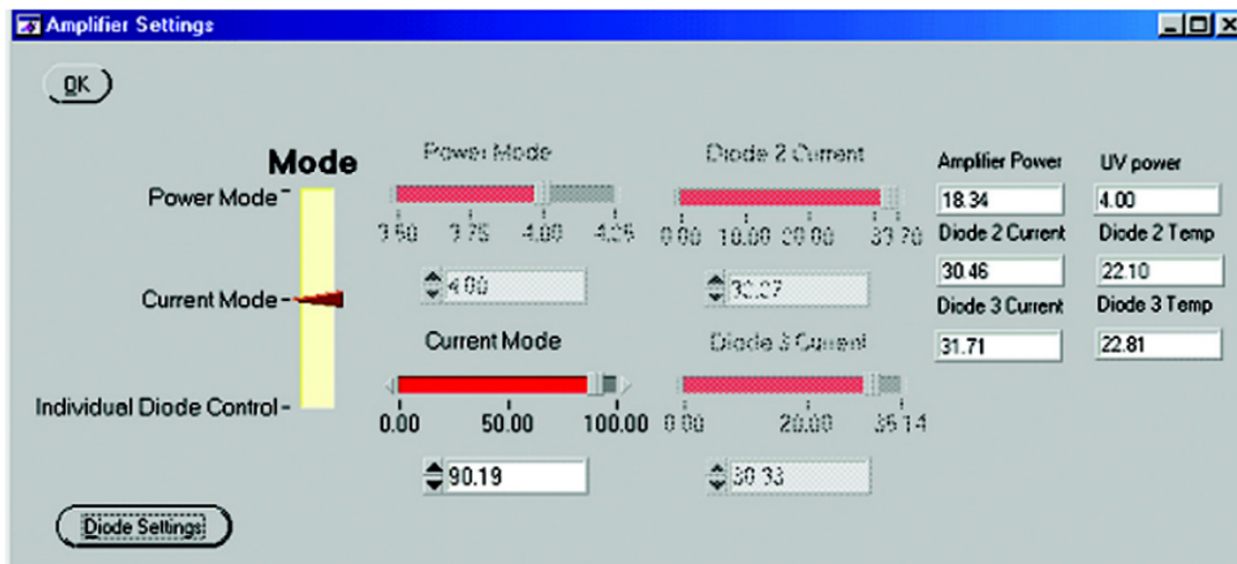
Figure 4.13: MLUV amplifier pump current control. In this figure the individual current controls are grayed out as the mode has not been set to individual diode control.
