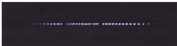
FIG. 1. Image of fluorescence from several trapped mercury ( ^{199}\text{Hg}^+ ) atomic ions. The ions are spaced by \approx 15 \mu\text{m} , and the two apparent gaps are different isotopes of mercury, which do not respond to the probe laser. (Courtesy of J. Miller and J. Bergquist, NIST)
