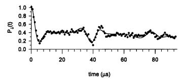
Figure 5.  $P_1(t)$  for a coherent state, driven on the second blue sideband. Since the Rabi frequencies are almost commensurate in this interaction,  $P_1$  shows very sharp collapse and revival features. The solid line is a fit using the exact Rabi frequencies for finite  $\eta$ . It yields  $\bar{n} = 2.0 \pm 0.1$ .
