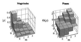
Figure 10. Experimental amplitudes  $\rho_{nm}$  and phases  $\Theta(\rho_{nm})$  of the number state density matrix elements of a  $|\beta| \approx 0.67$  coherent state. The state was displaced by  $|\alpha| \approx 0.92$ , for N=4 in equation (14).
