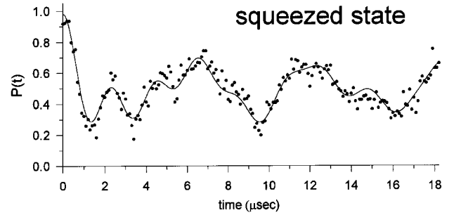
Figure 6. P_1(t) for a squeezed state. The data are fitted to a squeezed state population distribution, finding \beta \approx 40 \pm 10 (16 dB below the zero point variance), which corresponds to \bar{n} \approx 7.1 .
